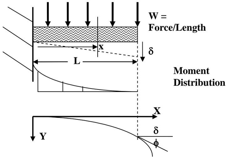
**Figure 1.11- A Beam under a Uniform Load**
