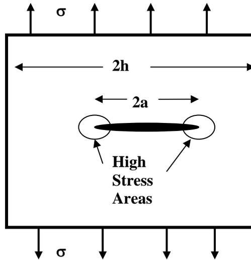
**Figure 3.3 – Crack Propagation in a Large Plane**
