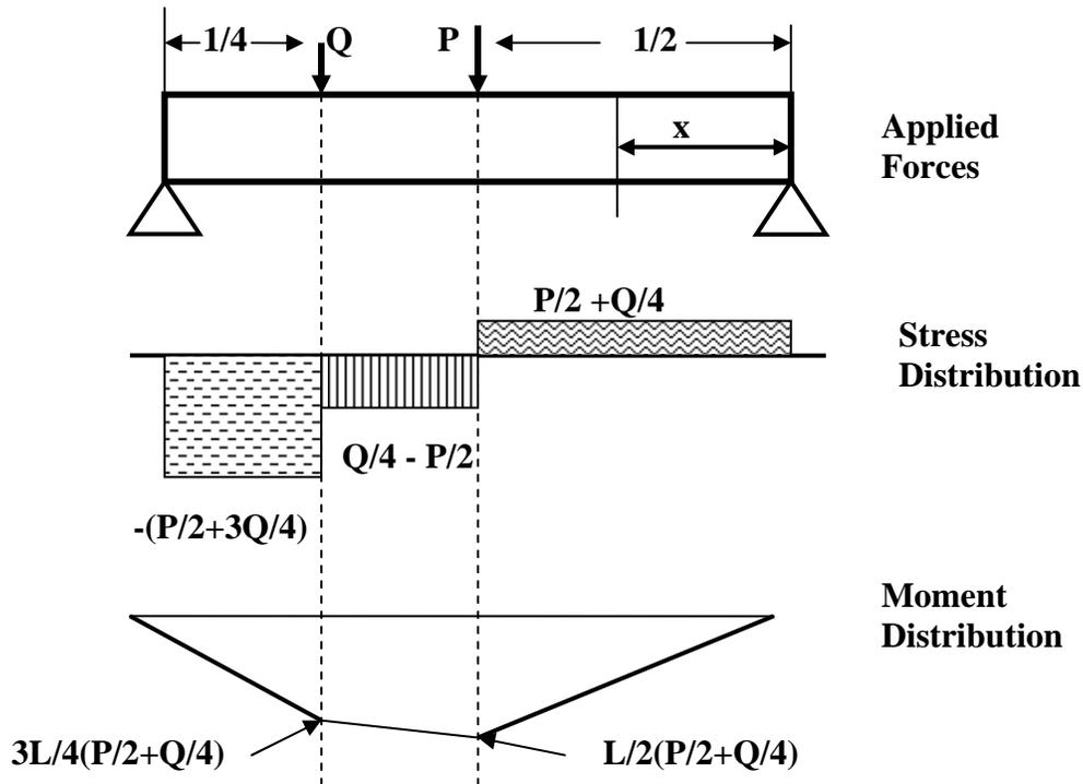
**Figure 1.9 – The Stress Distribution in a Beam**
