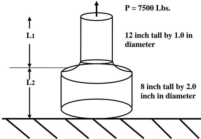
**Figure1.5 – A Tapered Shaft with a Load**
